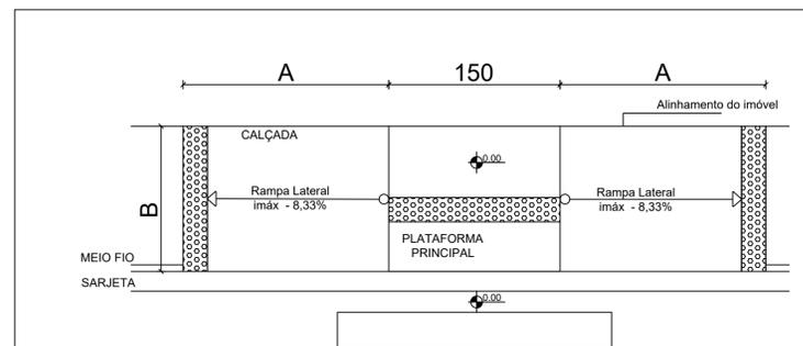
DETALHE - RAMPA - TIPO 1 SEM ESCALA
